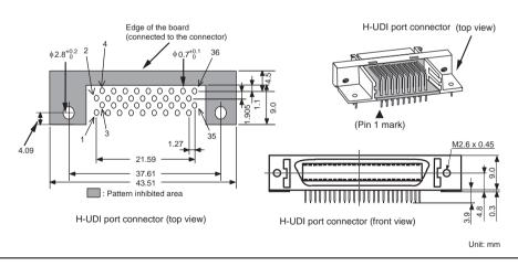
Figure 1.2 Pin Assignments of the H-UDI Port Connector (36 Pins)
